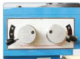
Vertical Spindle Speed Selectors
